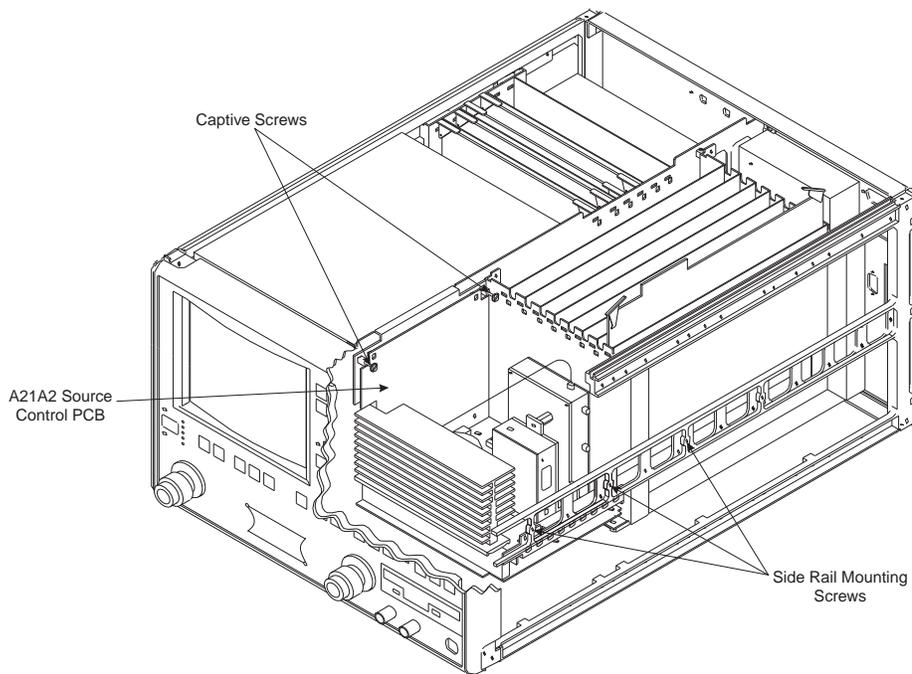
**Figure 8-10.** Signal Source Module Removal Details
