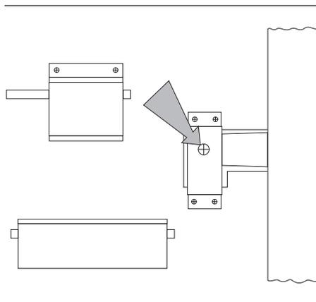
**Figure 8-4.** Removal of Test Set Module
