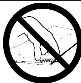
3. Do not handle static sensitive components in areas where the floor or work surface covering is capable of generating a static charge.
