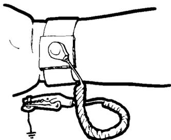
4. Wear a static-discharge wristband when working with static sensitive components.
