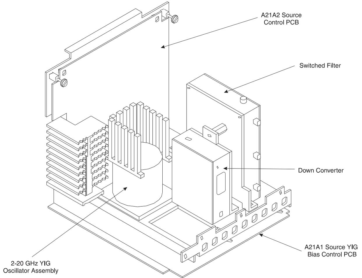
**Figure 2-2.** Signal Source Parts Location Diagram
