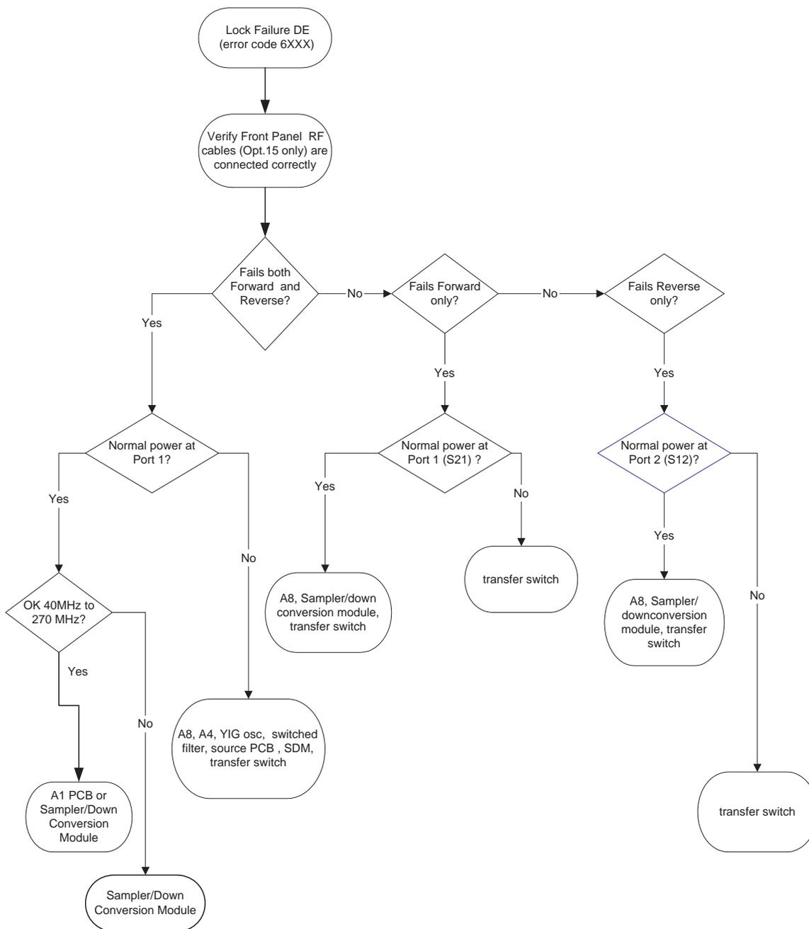
**Figure 7-3.** Error Code DE Lock Failure Troubleshooting (20 GHz and 40 GHz models only) (1 of 1)
