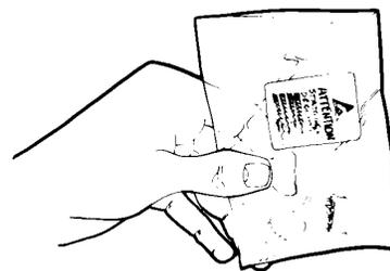
9. Transport and store PCBs and other static sensitive devices in static-shielded containers.
