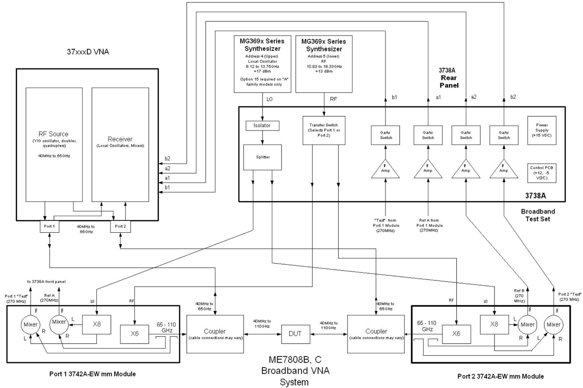
Figure D-1. ME7808B/C Block Diagram
