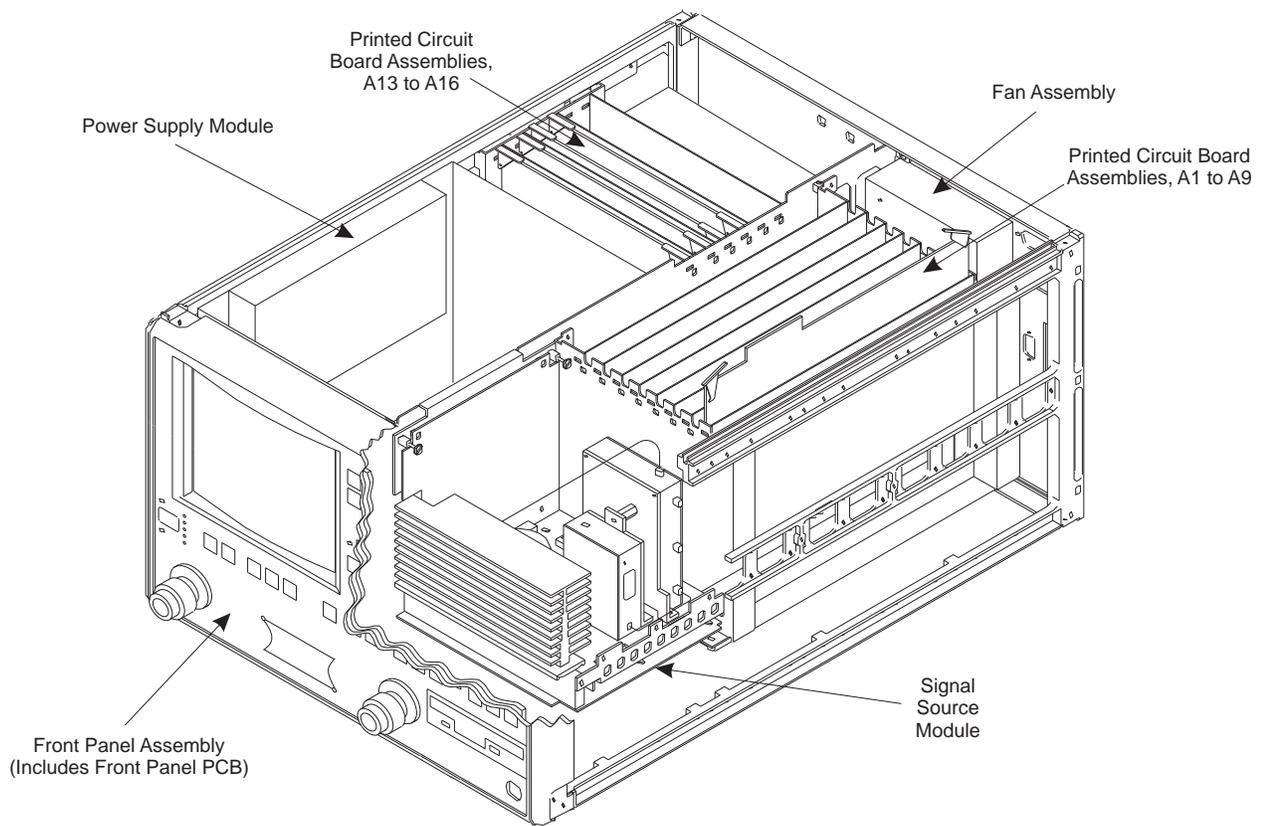
**Figure 2-1.** Major Assemblies Location Diagram (Top View)
