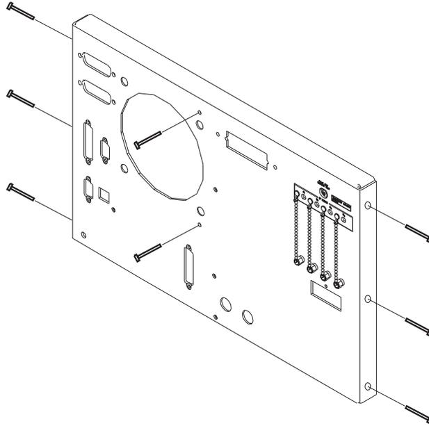
**Figure 8-6.** Rear Panel Mounting Screws
