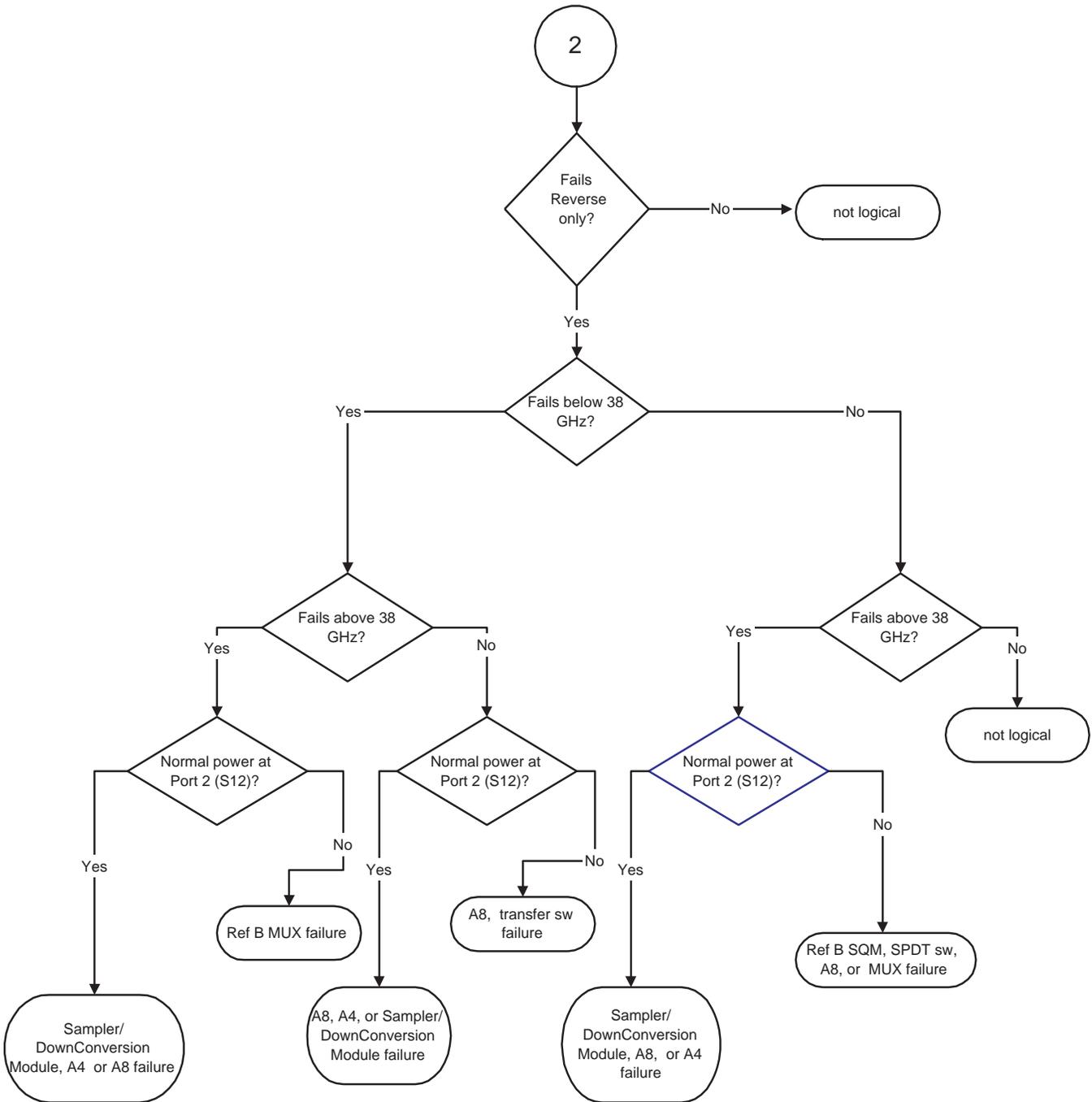
**Figure 7-2.** Error Code DE Lock Failure Troubleshooting (50 and 65 GHz models only) (3 of 3)
