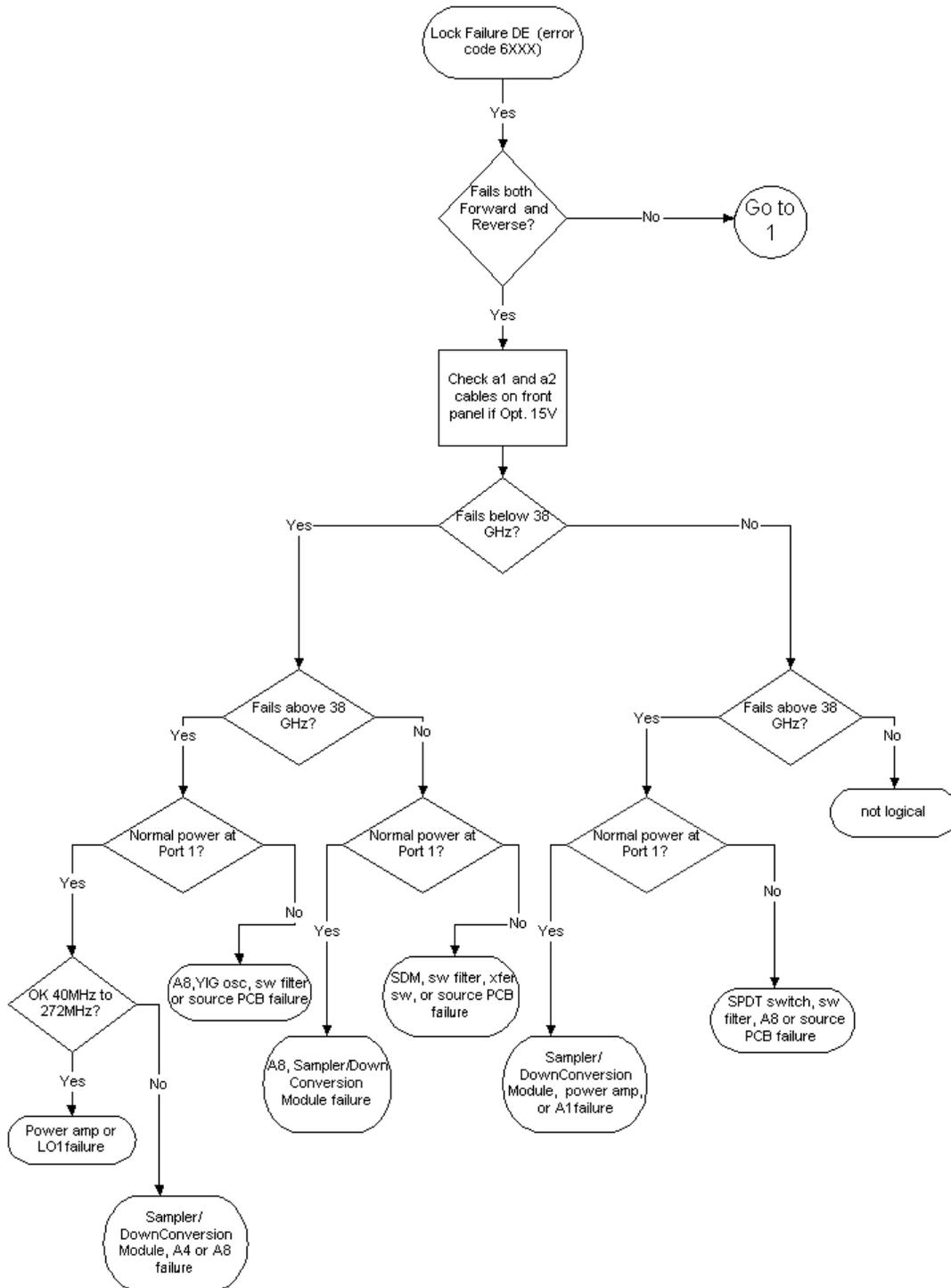
**Figure 7-2.** Error Code DE Lock Failure Troubleshooting (50 and 65 GHz models only) (1 of 3)
