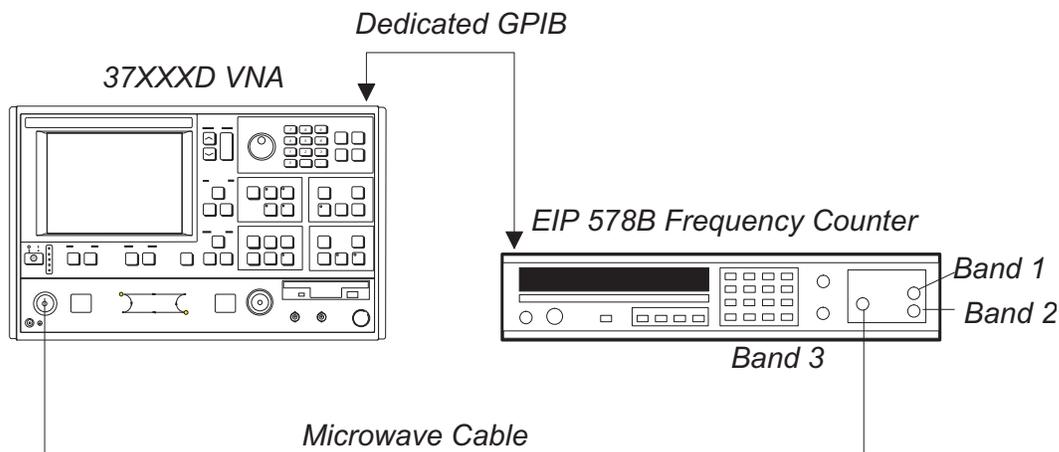
**Figure 6-1. Test Setup for Frequency Calibration**
