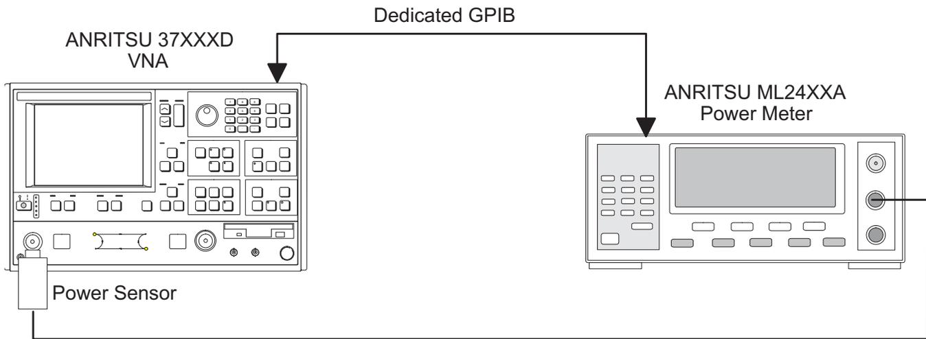
**Figure 6-2.** Equipment Set-Up for RF Power/ALC Calibration
