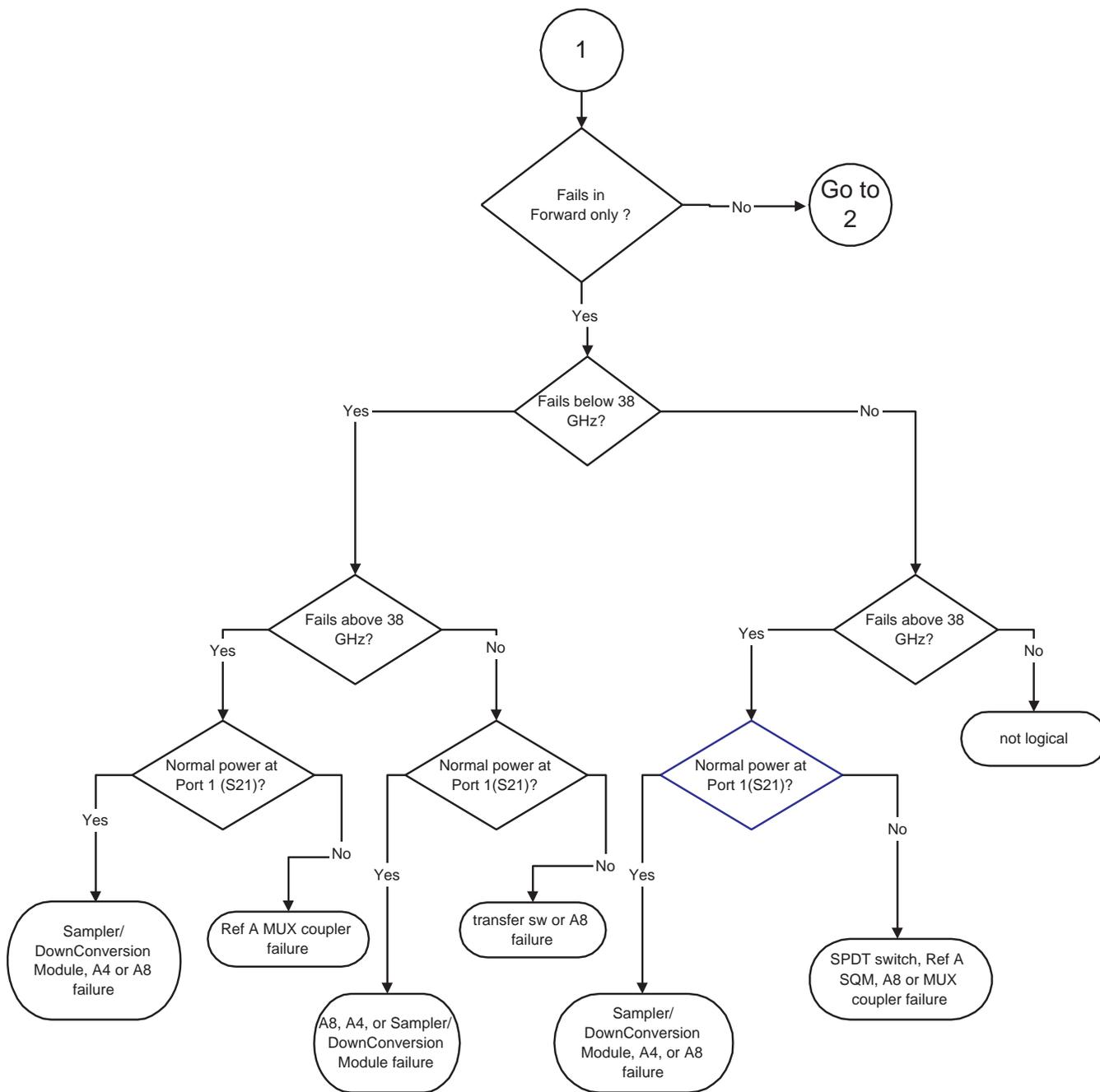
**Figure 7-2.** Error Code DE Lock Failure Troubleshooting (50 and 65 GHz models only) (2 of 3)
